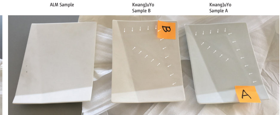
Linear markings on both plates that should not be there.
